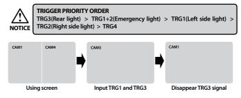
\* If the screen turns by trigger signal, [ 🕁 M 🚇 ] button doesn't wirk.
