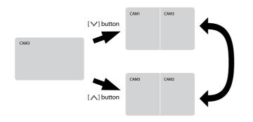
5) When there is input signal more than 2 triggers, the monitor display fully connected screen (Trigger input screen) as the priority order. And the screen goes former one when the signal is disappears, the rest will be display as the priority order.
